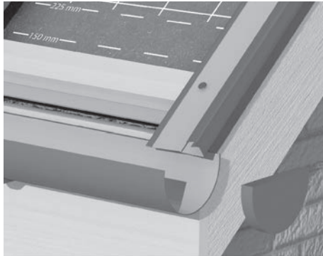
Fig. 19 – Nail each length of trim to batten
