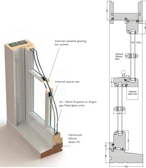
This is our highest specification range, designed to directly retro-fit in place of original box sash windows in older properties, or to create a traditional appearance in new-builds.
