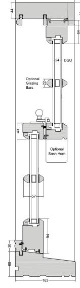
Featuring pre-tensioned spring balances in place of traditional weights and pulleys, these double glazed windows offer classic period styling combined with the latest timber window technology and skilled craftsmanship.
