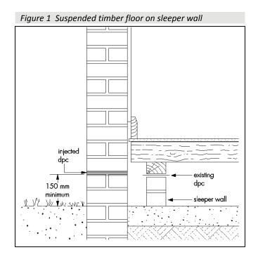
11.2 Where a suspended timber floor is supported on joists and/or a wall plate bearing on, or embedded in, the wall, there is a possibility of decay, particularly where concealed timbers are in contact with the damp wall. The condition of these timbers should be ascertained and remedial action taken if necessary (see Figure 2).
