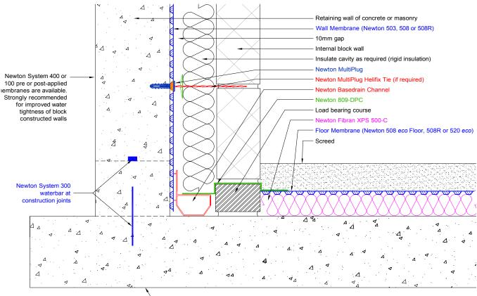
Newton 403 HydroBond is available a pre-applied bonded and self-healing sheet membrane to further waterproof the structure.
