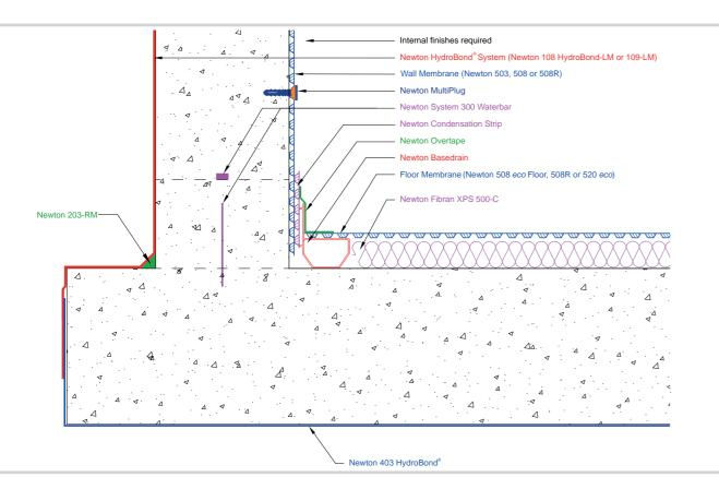
Newton HydroBond<sup>®</sup>, HydroTank and CDM Systems are employed to provide Type A, B & C waterproofing protection
