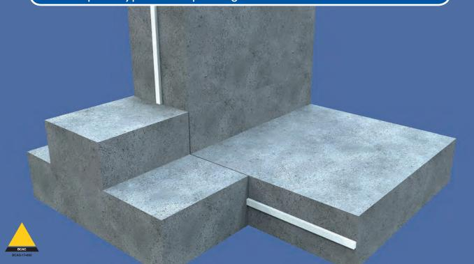
Newton 315 Polymer-Waterbar expands to seal water leaks through joints within the concrete to provide a Type B, water-resisting structure
