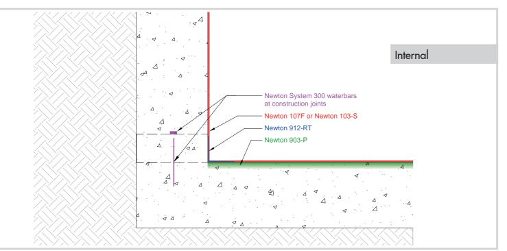
Type A internal waterproofing can be achieved by using a post-applied membrane such as Newton 107F or Newton 103-S. Both methods provide Type A barrier protection
