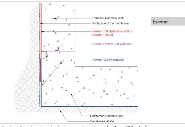
Type A protection can be achieved externally using a pre-applied membrane such as Newton 403 HydroBond<sup>®</sup>, or a post-applied liquid membrane such as Newton 108 HydroBond-LM or Newton 109-LM
