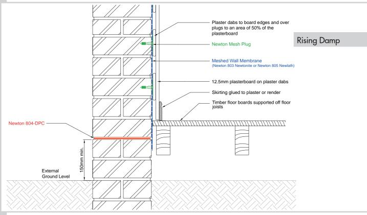
The Newtonite Damp Proofing System is the ideal solution to stop rising damp and allow for plaster finishes to be applied before the wall has fully dried out
