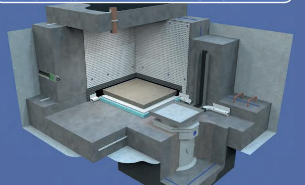
A typical combination waterproofing design showing the Newton CDM Cavity Drain System internally (Type C), Newton HydroBond<sup>®</sup> System externally (Type A), and the Newton HydroTank System incorporating waterbars and waterstops at weaknesses within the RC structure (Type B)
