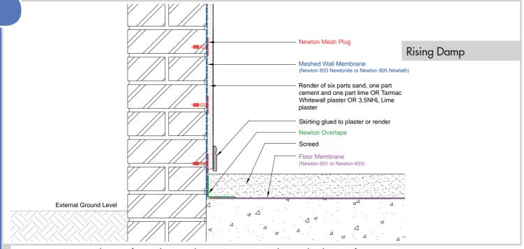
Newtonite damp proofing membranes, such as 803 Newtonite, provide a complete damp proofing solution when the wall and floor have been diagnosed with rising damp. The meshed surface provides a mechanical key for the direct application of plaster, render or dot and dab plasterboard
