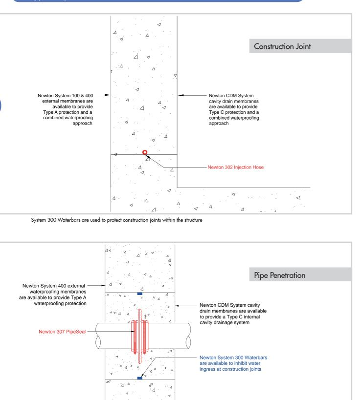
Newton 307 PipeSeal, applied through a new-build concrete wall using a "Box detail", prevents water ingress around a new service entry
