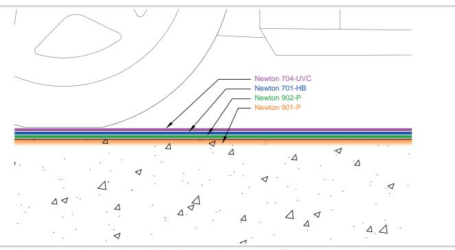
The Newton NewSeal system providing a highly durable, chemical-resistant, waterproof finish. The coating can be made anti-slip for external use and can be supplied in any RAL colour
