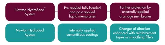
For internal application, cementitious coatings have tremendous grip and are therefore suitable for application to the "negative pressure" side of the structure. They can be applied by spray, trowel, brush or roller.
