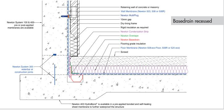
Typical detail showing the Newton CDM System with the Newton Basedrain channel within a formed recess
