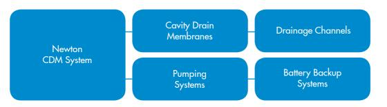
Often referred to as a 'water management system', water entering through the external walls of the structure is captured and depressurised in internal cavities that are created using drainage membranes and drainage channels. Now captured and stripped of its potency, the ingressing water can be safely removed from the building either by gravity to open elevations or by pumps.
