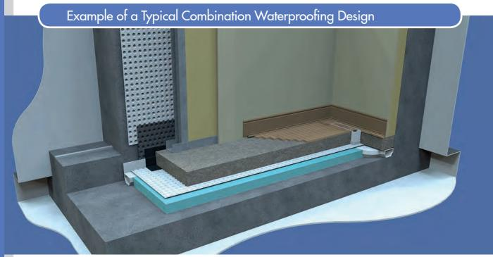
A typical combination waterproofing design showing the Newton CDM Cavity Drain System internally (Type C), Newton HydroBond $^{\circ}$  System externally (Type A) & Newton HydroTank for integral waterproofing details (Type B)
