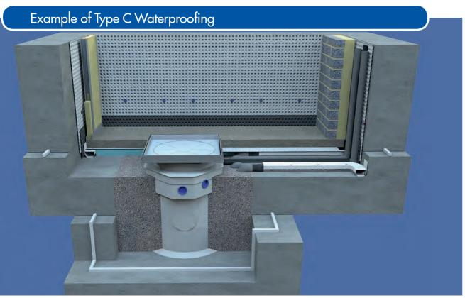
Newton cavity drain membranes are applied to the walls and floors, whilst Newton Basedrain channels collect water and provide drainage around the perimeter and above construction joints. Where removal by gravity is not possible, the Basedrain is connected to the Newton Titan-Pro pumping system to remove the water
