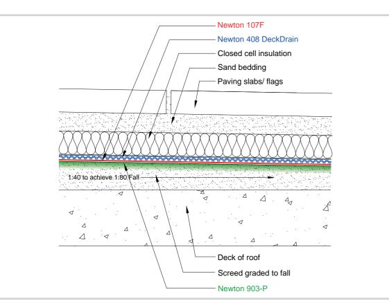
The Newton DeckFlex System providing waterproofing to an inverted warm roof specification to an RC concrete deck to protect the habitable space below
