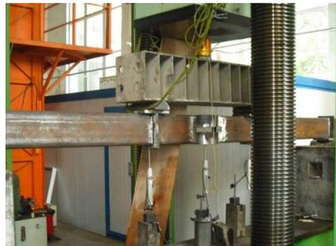
Fig. 9: Test Setup in Laboratory
