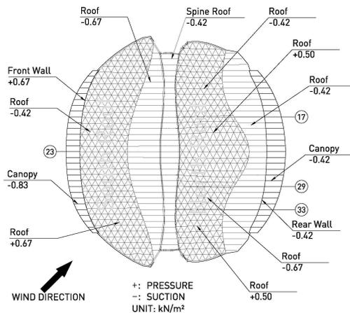
Fig. 14: Governing Wind Load Case for Global Stability
