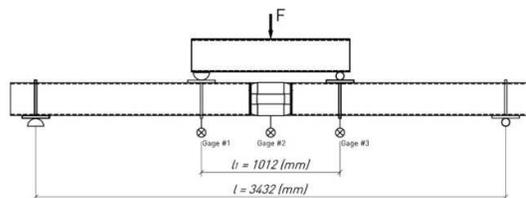
Fig. 8: 4-Point Bending Test Scheme
