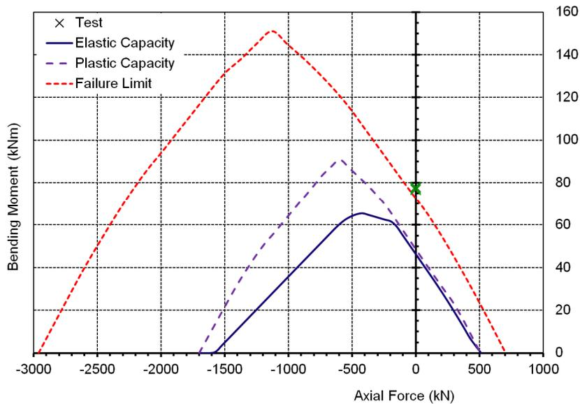
Fig. 12: Calculated Bending Moment Capacity vs. Axial Force
