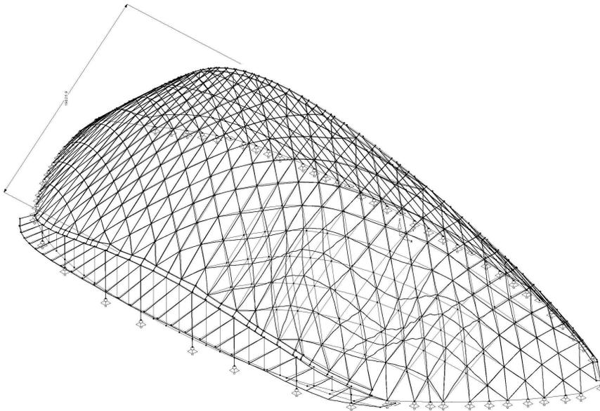
*Fig.15: First Global Buckling Mode of South Freeform Grid Shell*
