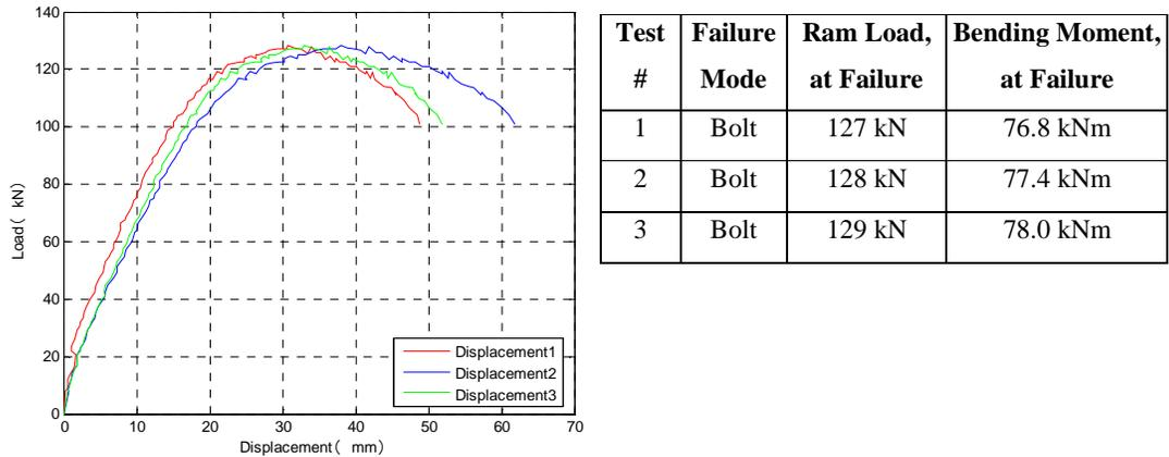
Fig.10: Ram Load - Displacement Curves Fig. 11: Bending Test Results
