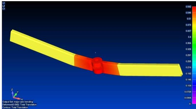
Fig. 13: Finite Element Model Displacements for 100 kN Test Ram Load
