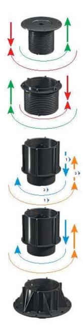
For heights greater than 120mm, series of towers are twisted into threaded colums on interior surface of baseplate and locked into place via termination clip on tower. Additional towers click into place on top of one another to increase height by 100mm each. Megapad Key (overleaf) used to unlock towers from baseplate.
