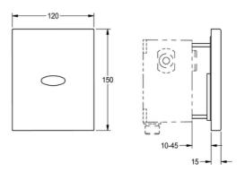
Finished installation kit for FLUSH-S non-touch, opto-electronically controlled urinal flush valve DN 15 for installation in walls. With self-closing solenoid valve cartridge, control electronics with sensor and stainless steel cover plate 120 x 150 mm.
