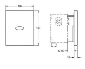
Finished installation kit for FLUSH-S non-touch, opto-electronically controlled urinal flush valve DN 15 for installation in walls. With self-closing solenoid valve cartridge, control electronics with sensor and stainless steel cover plate 120 x 150 mm.
