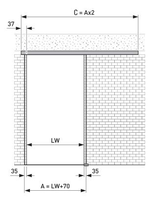
Ceiling and wall mounting, single door, complete sets for profile lengths up to 1996 mm (max. door width 975 mm) or 2996 mm (max. door width 1975 mm)
