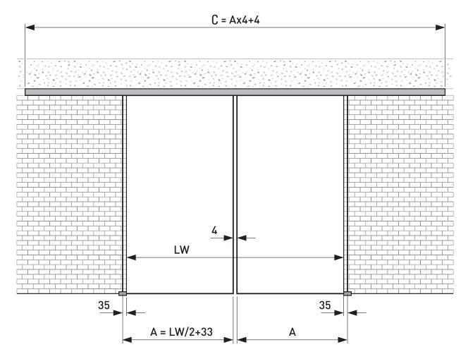
Ceiling and wall mounting, double doors, complete sets for profile lengths up to 3996 mm (max. width per door 975 mm) or 5996 mm (max. width per door 1975 mm)
