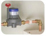
The hydraulic valve is an automatic urinal flush control valve. The valve uses a simple patented mechanism which prevents water waste by ensuring that the auto-flush cistern is only filled, and can only flush, when the washroom is used.
