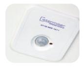
The infrared urinal flush control (IRC) valve automatically manages the supply of water to a urinal cistern. The PIR sensor detects movement and activates the solenoid valve allowing water into a urinal cistern.
