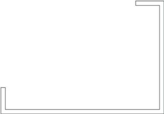
L shaped screens with double returns Can be made to any size to suit counter area up to 1500 x 1500 x 250 x 250
