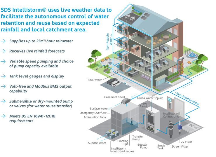
SDS WaterBank<sup>®</sup> Intellistorm<sup>®</sup> maximises the capacity for water reuse utilising only the attenuation volume, whilst minimising the potential for flooding by controlling the discharge of excess stored rainwater prior to a rainfall event.
