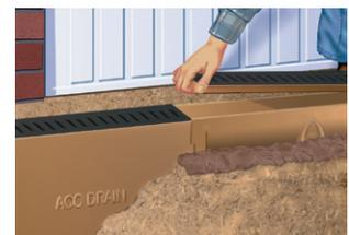
With gratings fitted, haunch around channels/sumps with concrete (suitable fill material). Final surface to be 3mm above grating. Bricks/paviours should be laid in mortar for lateral stability.
