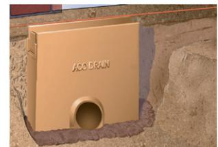
Knock out pre-formed outlet from the inside (marked with hammer symbol) or fit sump or outlet endcap. Position sump or outlet channel on concrete bed, fit PVC-U union/trap to drainage pipework.
