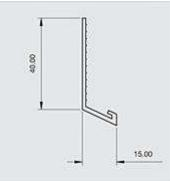
Locally manufactured from recycled plastic, Renderplas PVCu bellcast beads / drip beads are designed for function and speed on all external rendering applications. Discreet but strong, all beading gives a perfect finish to through colour render and is equally suitable for sand and cement
