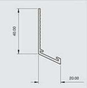
Locally manufactured from recycled plastic, Renderplas PVCu bellcast beads / drip beads are designed for function and speed on all external rendering applications. Discreet but strong, all beading gives a perfect finish to through colour render and is equally suitable for sand and cement
