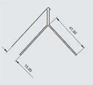
Locally manufactured from recycled plastic, Renderplas PVCu corner beads / angle beads are designed for function and speed on all external and internal rendering and plastering applications. Discreet but strong, all beading gives a perfect finish to through colour render and is equally suitable for sand and
