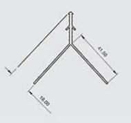
Locally manufactured from recycled plastic, Renderplas PVCu corner beads / angle beads are designed for function and speed on all external and internal rendering and plastering applications. Discreet but strong, all beading gives a perfect finish to through colour render and is equally suitable for sand and cement
