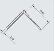
Locally manufactured from recycled plastic, Renderplas 2mm PVCu arch corner beads / angle beads are designed for external and internal arches to provide protection from impact and speed up application for a smooth regular curve on the outer edge
