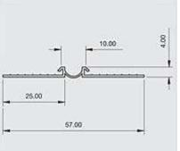
Locally manufactured from recycled plastic, Renderplas PVCu movement joint / expansion joint beads are designed for areas of render over 20 square metres and should be specified every 4-6 metres, over structural movement joints and changes of background giving a discreet attractive finish. Also for use as an internal corner with plasterboard
