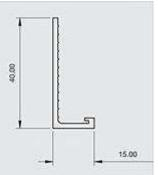
Locally manufactured from recycled plastic, Renderplas PVCu stop beads are designed for function and speed on all external and internal rendering and plastering applications. Discreet but strong, all beading gives a perfect finish to through colour render and is equally suitable for sand and
