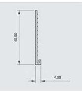
Locally manufactured from recycled plastic, Renderplas PVCu stop beads are designed for function and speed on all external and internal rendering and plastering applications. Discreet but strong, all beading gives a perfect finish to through colour render and is equally suitable for sand and cement
