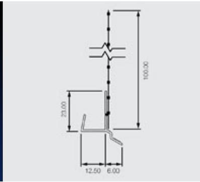
Renderplas PVC 12.5mm board casing bead with integrated 6mm drip and 100mm glass fibre reinforcement mesh. Combination edge bead and drip bead for render carrier boards, cement boards and Aqua Panels
