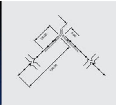
Renderplas PVC 6mm corner /angle beads with glass fibre reinforcement mesh are designed for function and speed on all EWI and thin coat rendering applications
