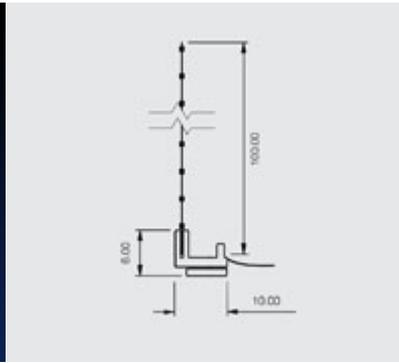
Renderplas PVC reveal beads with integrated foam vibration strip and glass fibre reinforcement mesh. Designed to protect frames and surfaces in reveals and extend the life of render and EWI systems
