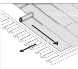
The alkorPLAN® roofing membrane has two lines printed along the edge during the manufacturing process. The first line is the centre line for the fasteners and the second line is the extent of the overlap of the adjacent sheet of alkorPLAN®. This is known as the weld line.
