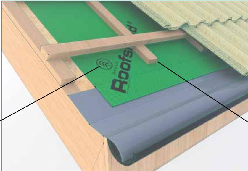
Roofshield fully supported on insulation
