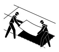
Where Servipak boards abut the parapet, pipe bays or abutments they should be pre-measured, and accurately cut to size by incising with a sharp knife and breaking on edge. The joints between the Servipak boards should be dry and primed with Primer B2.
