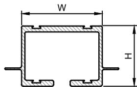
Aluminium track with ceiling support angle 'B'
