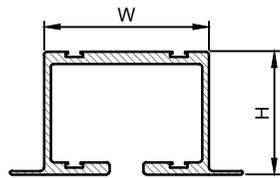
Aluminium track with ceiling support angle 'A'
