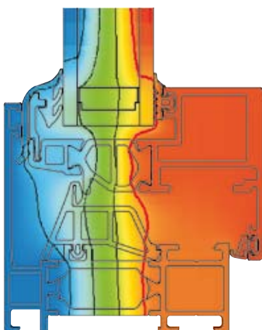
Schüco AWS 65 BS High levels of thermal insulation thanks to hollow chamber insulating bar and multi-chamber centre gasket
