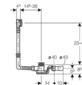
**Geberit bath drain with push actuation PushControl**
