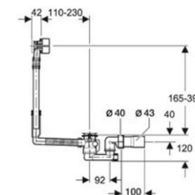
**Geberit bath drain with turn handle actuation and inlet**
