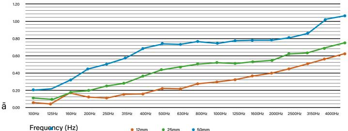
Sound absorption @ 12mm (Random Incidence) NRC > 0.27 Sound absorption @ 25mm (Random Incidence) NRC > 0.42 Sound absorption @ 50mm (Random Incidence) NRC > 0.67
