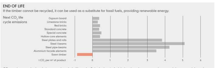
$CO_2$  can be saved using timber over the whole life cycle. Substituting  $1m^3$  of timber for other construction materials can result in savings of up to 1 tonne of  $CO_2$ . This combined with the carbon storage, means that  $1m^3$  of timber stores and substitutes 2 tonnes of  $CO_2$ .
