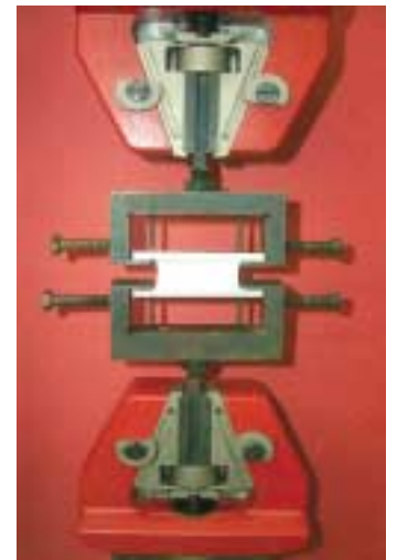
Sikaflex ® sealant undergoing extension and compression testing to B.S.9047 courtesy of Oxford Brookes University
