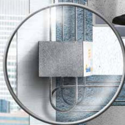
*Designing parapets to Passive House standard is a particularly demanding challenge and the Schöck Isokorb® type AXT offers just the right solution. Which is why it is the only load bearing thermal insulation element for parapets to have been certified by the Passive House Institute in Darmstadt.*
