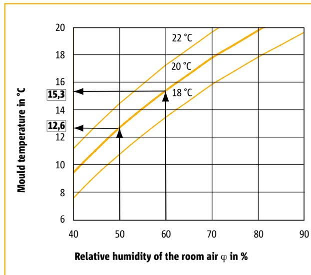
Figure 32: Dependency of the mould temperature on the room air humidity and temperature.
