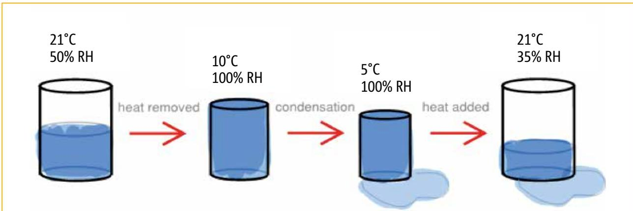
Figure 30: Illustration of condensation process.
