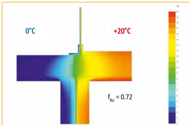
Figure 14a: Balcony connection without thermal breaks: temperature distribution (section). This detail does NOT conform to UK Building Regulations Part L requirements for minimum temperature factor in dwellings ( $f_{Rsi} = 0.75$ )
