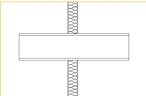
Figure 23a: HEA200 beam passing through 80mm insulation
