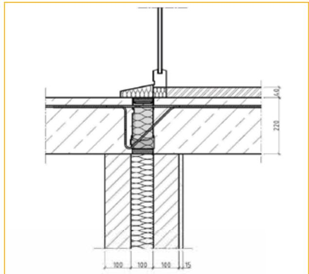
Figure 13b: Schöck Isokorb® type K50 installed in construction.
