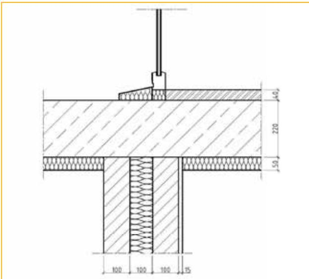
Figure 13a: Wall construction with balcony slab through.
