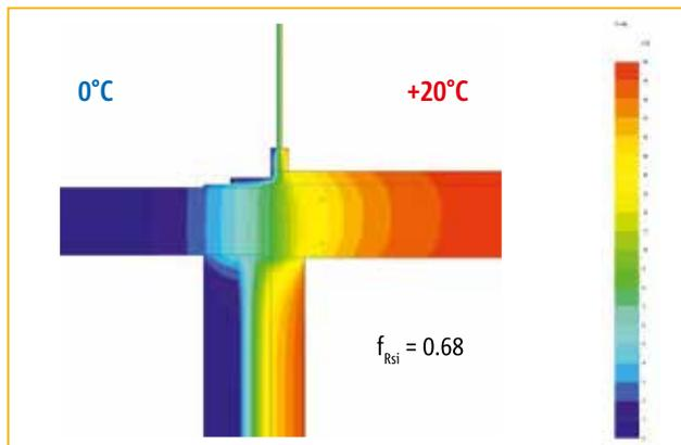
Figure 19a: Direct connection (Case 1): temperature distribution (section) This detail does NOT conform to UK Building Regulations Part L requirements for minimum temperature factor in dwellings ( $f_{Rsi} = 0.75$ )
