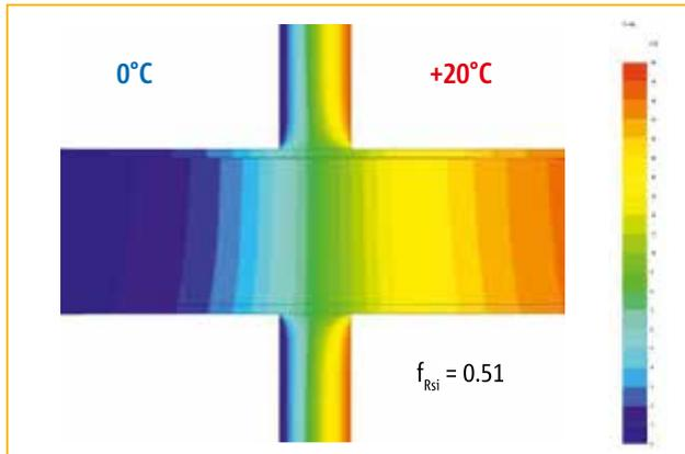
Figure 24a: Direct connection (Case 1): temperature distribution (section)
