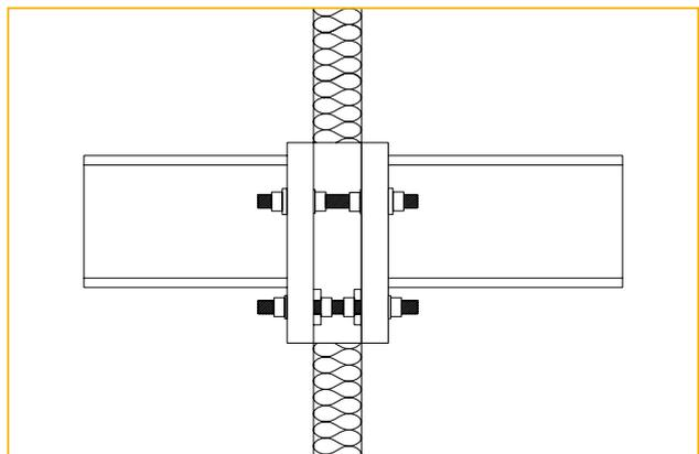
Figure 23b: Thermally broken steel beam with KST22
