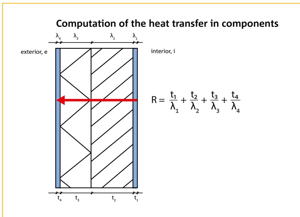
Figure 26: A representation of a wall construction, to define the  $R$  value by the thickness of the layers and the corresponding  $\lambda$  value.
