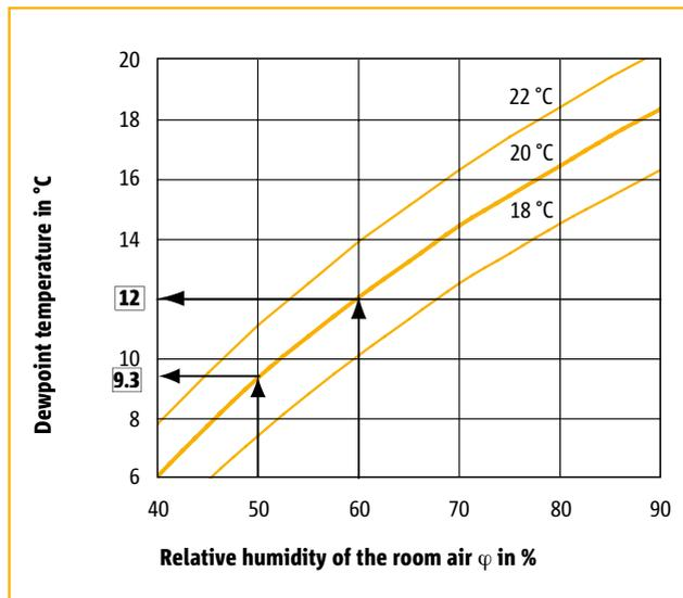
Figure 31: Dependency of the dewpoint temperature on the room air humidity and temperature.
