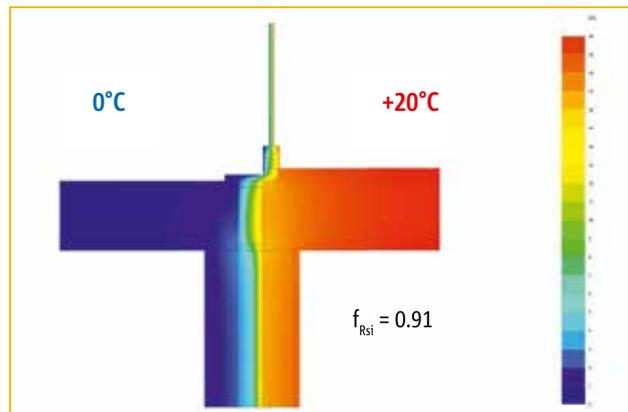
Figure 14b: Schöck Isokorb® type K50 connection: temperature distribution (section). This detail conforms with UK Building Regulations Part L requirements for minimum temperature factor in dwellings ( $f_{Rsi} = 0.75$ )
