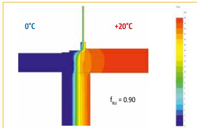
Figure 19b: KS14 H200 connection (Case 4): temperature distribution (section). This detail conforms with UK Building Regulations Part L requirements for minimum temperature factor in dwellings ( $f_{Rsi} = 0.75$ )
