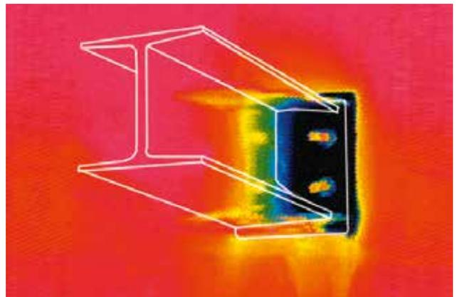
Figure 11: Thermal bridging occurring at continuous steel beams.
