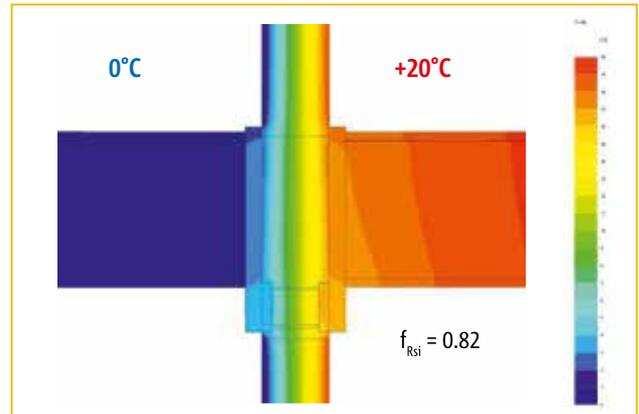
Figure 24b: KST16 connection: temperature distribution (section). This detail conforms with UK Building Regulations Part L requirements for minimum temperature factor in dwellings ( $f_{Rsi} = 0.75$ )
