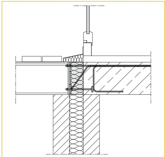
Figure 18b: Schöck Isokorb® type KS14 installed in construction.
