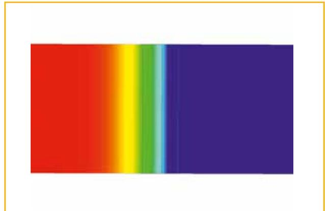
Figure 8b: Top view; this shows a cross-section through the balcony slab presented in 8a. You can clearly see that the heat loss is linear, meaning it remains the same across the entire connection length of the balcony.
