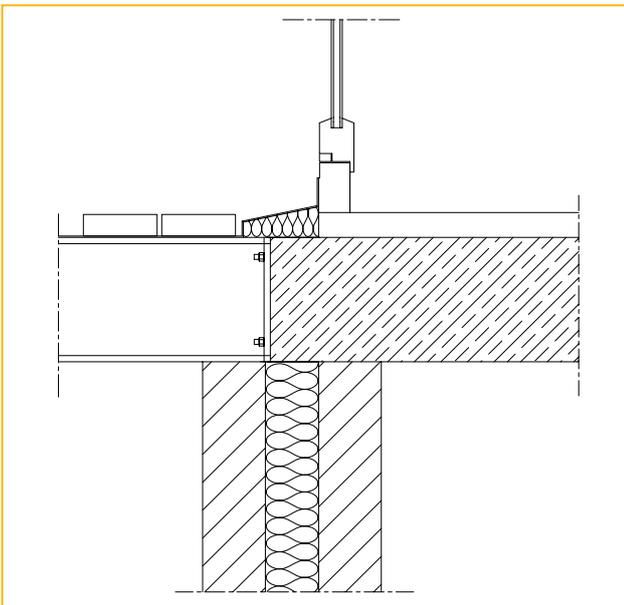
Figure 18a: Wall construction with a direct steel balcony connection.
