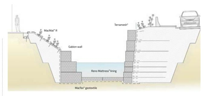
The channel banks may also be unstable and require structural support; our retaining walls and soil reinforcement solutions, appropriately designed and specified for use in a fluvial environment are ideal.
