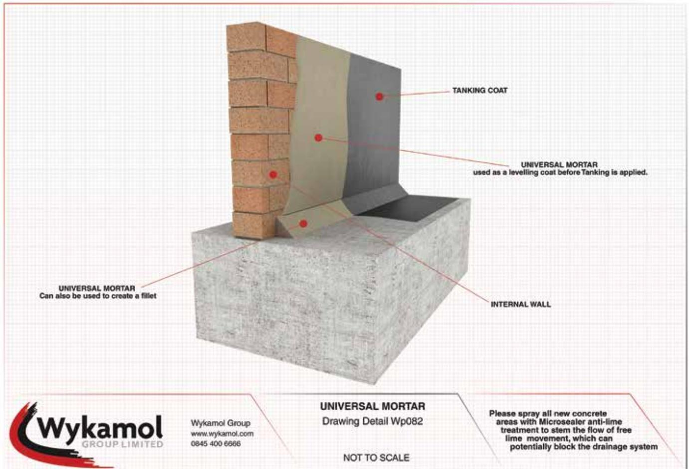
into the chase at the wall/floor joints and joints at the wall/wall. Whilst still green, form a “bottle” cover and feather for 50 - 100 mm along the adjacent surfaces. Achieve a smooth finish to the fillet.
