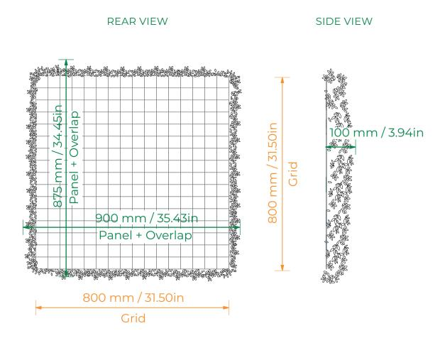
Vistafolia®'s Panels were designed with a small allocation of 'planting overlap' to allow for seamless installation of multiple panels. The top overlap is slightly greater than the bottom one whereas the side overlaps are the same. The overlap also serves to disguise the grid that holds the plants.
