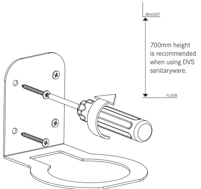
Mark and fix the cistern bracket to the appropriate height using suitable fixings (not supplied).
