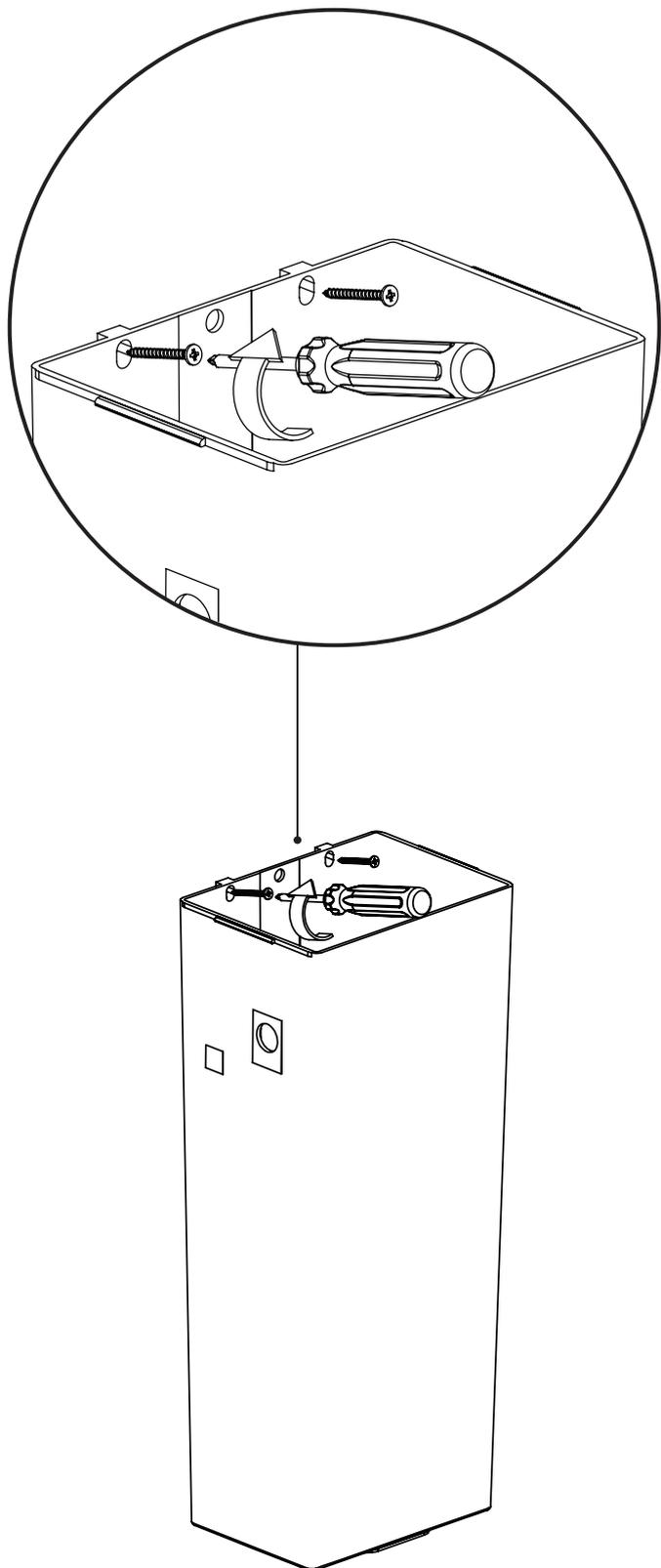
Mark through the 2 outer pre-drilled holes located in the back of the cistern, now secure using suitable fixings (not supplied).
