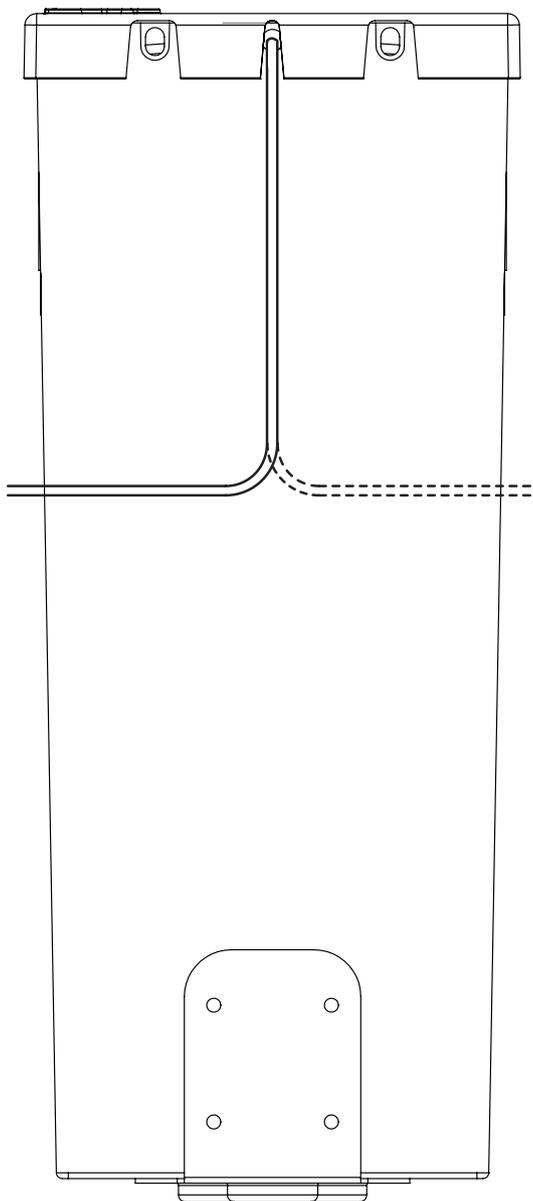
Position the base of the cistern on to the bracket fixed in the previous step, now ensure the flushvalve cable trails downwards **only** and exiting to the left or right (as above).
