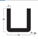
For framing glass panels, for edge protection or for all-glass constructions and diverse applications  $\cdot$  minimum surface roughness, exquisite-looking finish
