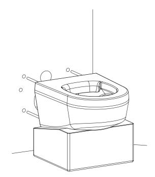
Screw the M12 studding into the back of the pan as far as possible. Make sure a flush pipe cone and outlet connector is fitted in the back of the pan. The cradle can be used to support the pan. Allign the pan with fixing holes.
