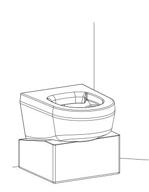
Using the cradle, slide the pan into place against the wall so all the fixing studs protrude through into the service duct.
