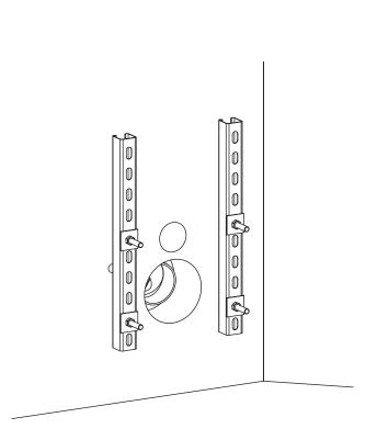
Secure the pan to the wall using the nuts and washers supplied- tighten using a torque wrench to 22-24 Nm. Connections to the WC flush pipe and soil pipes are conventional.
