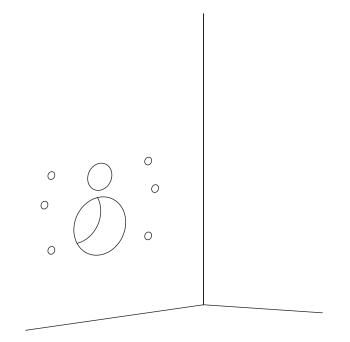
Use the drilling template provided, mark and drill holes for the inlet, waste and fixing studding. For disabled use, raise hole heights an additional 60mm.
