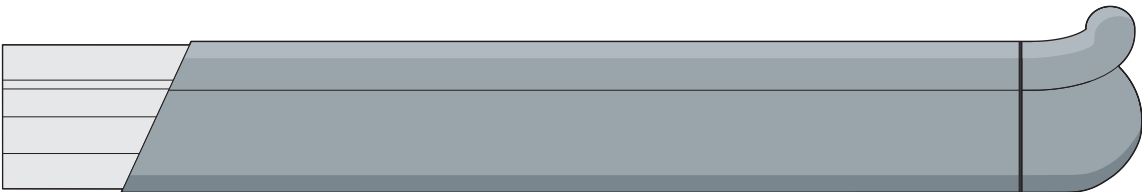
CHR110 continuous aluminium retainer with PVC-u cover
