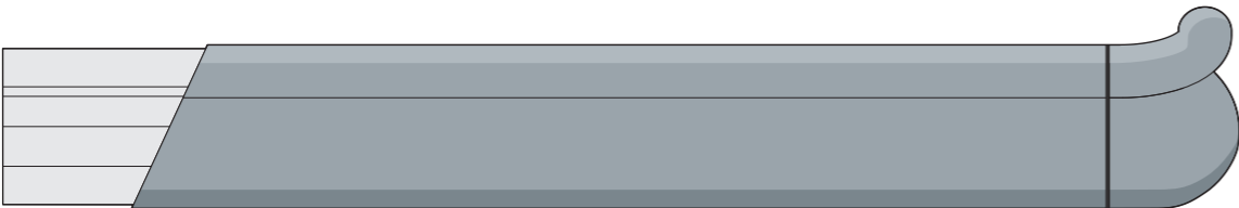
CHR110 continuous aluminium retainer with PVC-u cover
