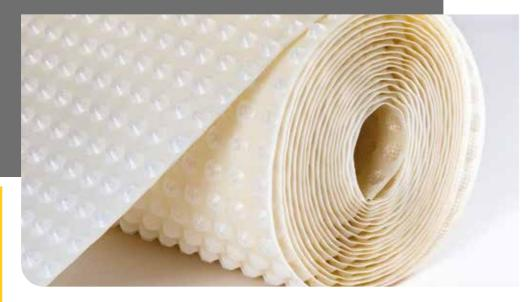
CM8 Cavity Drain Mesh Membrane is a 8 mm studded membrane incorporating a tough HDPE mesh lathing welded to the front face, allowing the direct application of various plaster finishes, adhesive 'dabs' and plasterboards and delivering a grade 3 environment to BS8102:2022 and NHBC Chapter 5.4
