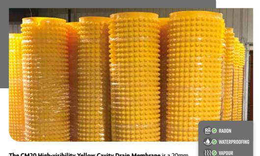
The CM20 High-visibility Yellow Cavity Drain Membrane is a 20mm studded membrane, suitable for Type C waterproofing and delivering a grade 3 environment to BS8102:2022 and NHBC Chapter 5.4. CM20 Yellow is the highest drainage capacity membrane in the Wykamol Waterproofing range.
