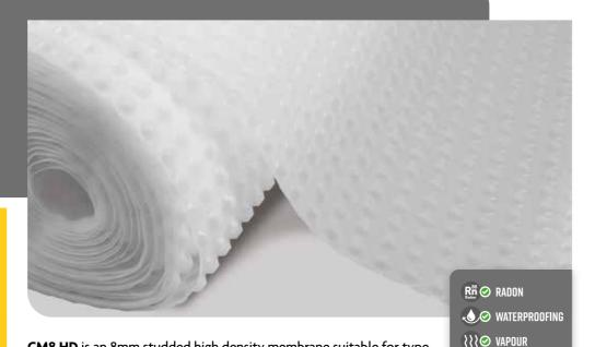
CM8 HD is an 8mm studded high density membrane suitable for type C waterproofing and delivering a grade 3 environment to BS8102:2022 and NHBC chapter 5.4. We recommend using the HD version on our insulated spacer and also in commercial areas where a more impact resistant membrane may be needed. CM8 HD is also an excellent Radon barrier and has passed all the relevant tests for resistance to this Gas.
