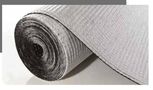
Wykamol geotextile 8 and 20mm membrane is a 2 metre wide pre-formed drainage waterproofing and gas venting solution, providing a sustainable, environmental alternative to traditional filter stone drainage layers.
