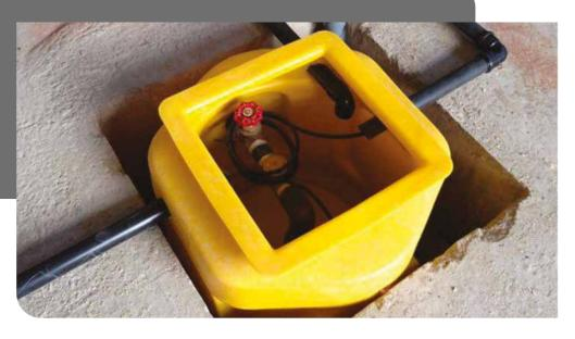
The system comprises of a polyethylene tank, locking access cover (pedestrian duty, not suitable for roadways) and powerful submersible pump. The system is very versatile, enabling the installer to locate inlets to their specifications. The system comes complete with a High Level Alarm (9V), which acts as a warning system to alert the end user if the water rises above the normal operating level.
