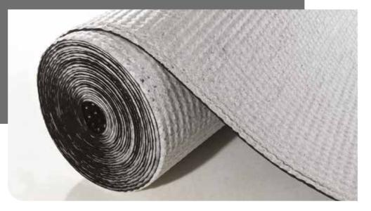
The dual layers comprise of the Wykamol 8mm studded HDPE membrane and a non-women geotextile manufactured from UV stabilised, virgin polypropylene fibres that have been mechanically entangled to provide high strength, high extensibility, high loft and excellent abrasion characteristics. The geotextiles are also thermally treated to reduce thickness while maintaining excellent mechanical properties.
