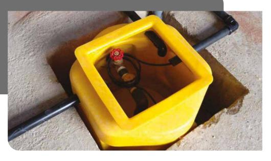
The system comprises of a polyethylene tank, locking access cover (pedestrian duty, not suitable for roadways) and powerful submersible pump. The system is very versatile, enabling the installer to locate inlets to their specifications. The system comes complete with a High Level Alarm (9V), which acts as a warning system to alert the end user if the water rises above the normal operating level.
