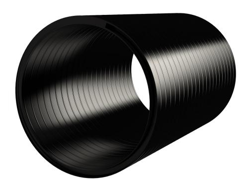
The uniqueness of the Weholite production process means that pipes can be run in any length from 300mm to 30m in one piece. It is one of the few polyethylene pipes in the world that can be produced in dimensions larger than two metres and can be supplied in ring stiffness classes from 2 to 8kN/m<sup>2</sup>.
