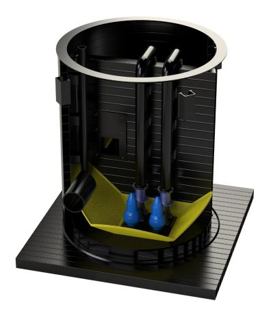
These systems are manufactured to varying depths and fully assembled in the factory with all the internal pipework and valves. The modular system simplifies the installation process, reducing overall cost whilst ensuring each assembly is functioning correctly.
