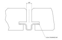
Dimensions Weight Density Flexural strength Point load@400 ctrs Point load@300 ctrs Distributed load@400 ctrs Distributed load@300 ctrs Finish Fire performance 150 x 2440 x 25mm 5.95kg / Im 38.4kg / m2 1.5g/cm3 20MPa >3KN as per BS EN 1991-1-1 >4KN as per BS EN 1991-1-1 >4KN as per BS EN 1991-1-1 >5KN as per BS EN 1991-1-1 Matt wood grain Euroclass Al to EN 13501
