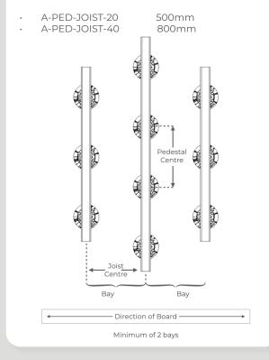
ZERODECK: 6.45 linear metres per m2 Joists: 1.67 linear metres per m2, Clips: 15 per m2. Costs exclude pedestals - allow 4 pedestals per m2. Exact pedestal numbers will depend on site-specific requirements including finished floor level and falls.
