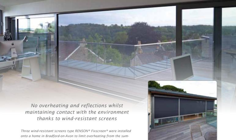
mer sun. These external roller blinds stop the sun's rays from contacting the glass whilst still allowing the occupant to see outside.
