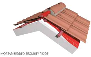
Mechanical fixing system for mortar bedded ridge ridges, helping house builders and contractors meet British Standards and NHBC guidelines.
